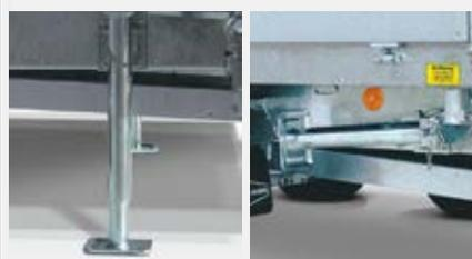
**Double the stability:** Swivelling, removable telescopic crank drop legs.
