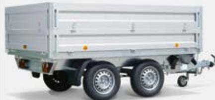
**More space:** The anodised aluminium box attachment increases the height of the sidewalls and doubles the loading volume\*\*.
