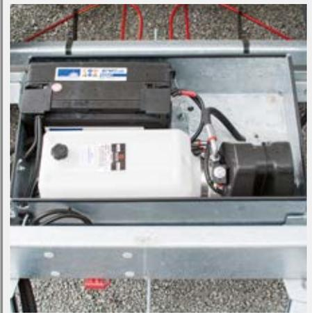
**Time is money:** Loose materials are unloaded quickly and conveniently with the electric hydraulic pump with emergency hand pump (accessories, see page 13).
