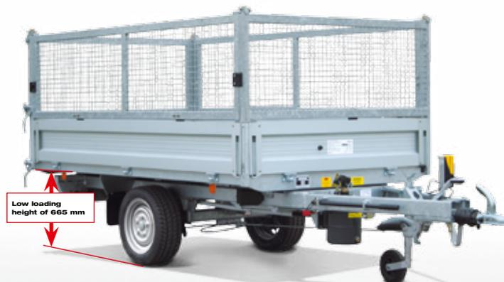
**More comfort:** The impressive RK-AL 2514 has an extremely low loading height of 665 mm as well as a low centre of gravity that optimises the handling characteristics of the trailer and increases driving safety as a result. The steel mesh attachment (accessory) prevents lightweight materials from blowing away (electronic hydraulic pump with remote control and emergency hand pump; accessories).
