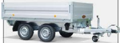
**Transport more:** The robust anodised raised aluminium sidewalls, reinforced in a closed profile, create more space for your load\*\*.
