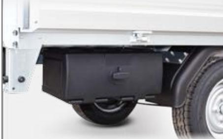
**Storage space for important tools:** With generous dimensions (440 x 150 x 210 mm) and a max. load capacity of 20 kg, the extremely spacious storage box can also be locked (available for the RK-AL 2514, DK-AL 3218 and DK-AL 3718 models).
